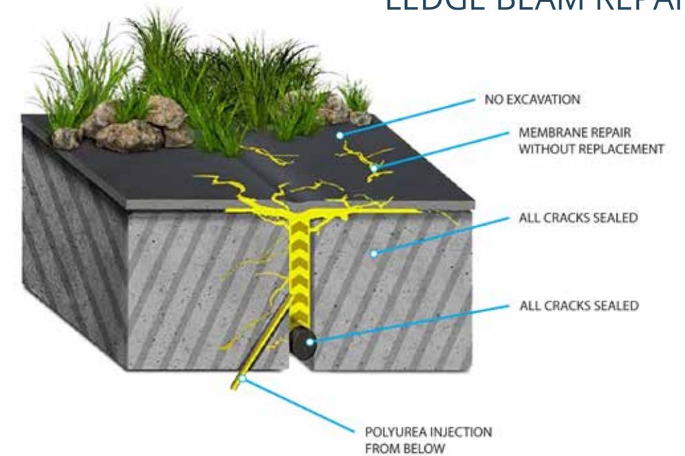
Negative-side injection (from inside the parking garage) saves time and costs: no excavation or membrane removal are needed – less labour is used. The areas repaired are reopened for use in less than 24 hours.
